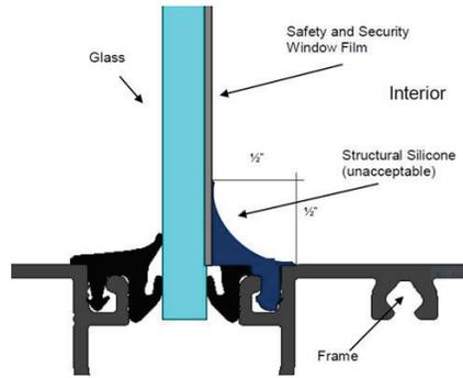
Curing time for the silicone depends upon temperature and humidity. Do not clean the film or frame for at least 30 days following installation of the silicone. Full cure of the silicone should occur within 30 days following installation.
