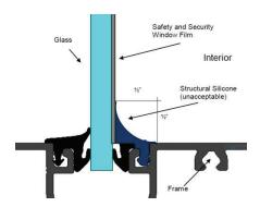
Curing time for the silicone depends upon temperature and humidity. Do not clean the film or frame for at least 30 days following installation of the silicone. Full cure of the silicone should occur within 30 days following installation.
